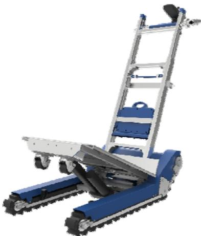
The CT420 can walk on flat ground with crawler tracks. Switch to the loading board manual operation mode, raise the loading board to an angle till the crawler tracks touch the ground, and then the operator can move the machine by controlling the joystick.
