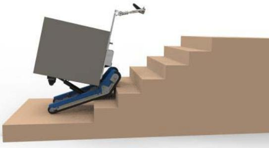
**When CT420 goes downstairs to the last three stairs, automatic loading board adjustment mode is recommended, set speed to 1. Turn to loading board automatic adjustment mode by handheld controller. If the manual adjustment mode is applied please make sure the balance of the loading board, shift between the track walking mode and manual adjustment mode. And when the tracks land on the floor, the floor walk mode can be launched.**
