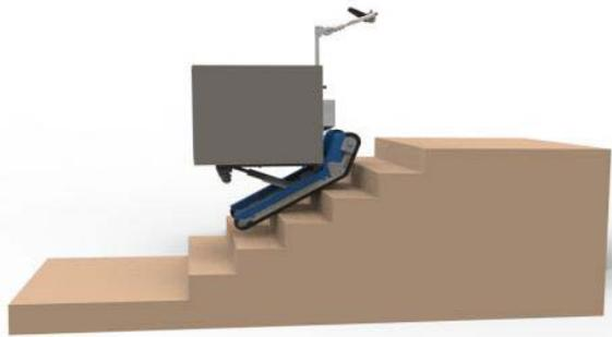
**When CT420 gets off the edge of the platform totally and goes down stably, cancel automatic mode. If the base of CT420 is unstable when going downstairs, adjust to rotating mode by handheld controller. Adjust manually loading board rotating angle according to different cargo gravity so that CT420 can go downstairs stably. Then the speed can be increased.**
