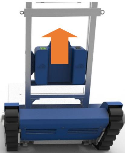
**2、 Remove the battery in the arrow direction shown in the picture.**
