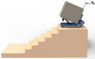
**Make sure the goods is fixed securely, move CT420 to the edge of the stairs and make sure two crawler tracks lean against the edge of the first stair. Turn on loading board automatic mode by handheld controller, set to speed 1, and go down under track moving mode.**
